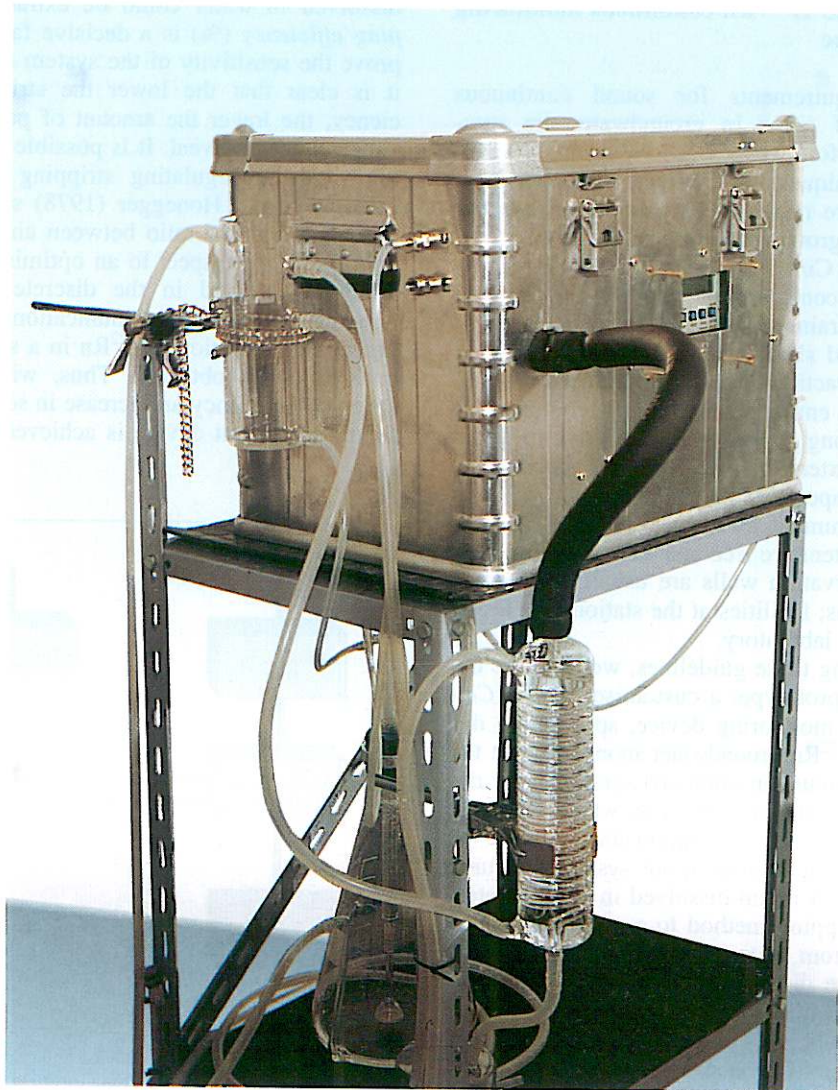
Fig. 1b. Photograph of the final assembly of the ING radonmeter prototype.
