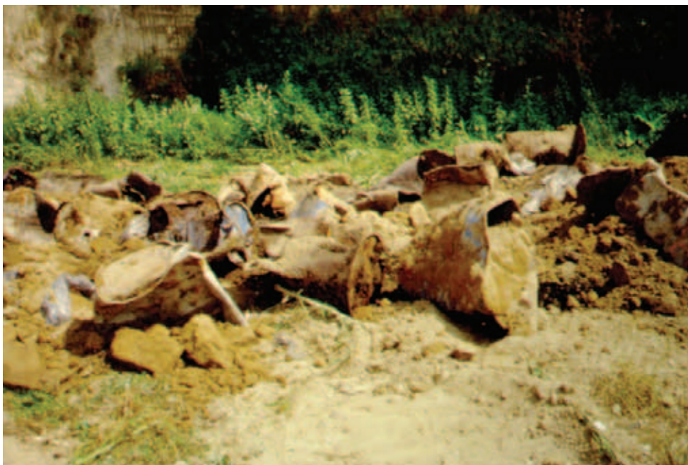
Photo 1. Some steel drums dug out after the first magnetometric survey performed at Riano Flaminio (north of Rome, Italy).
