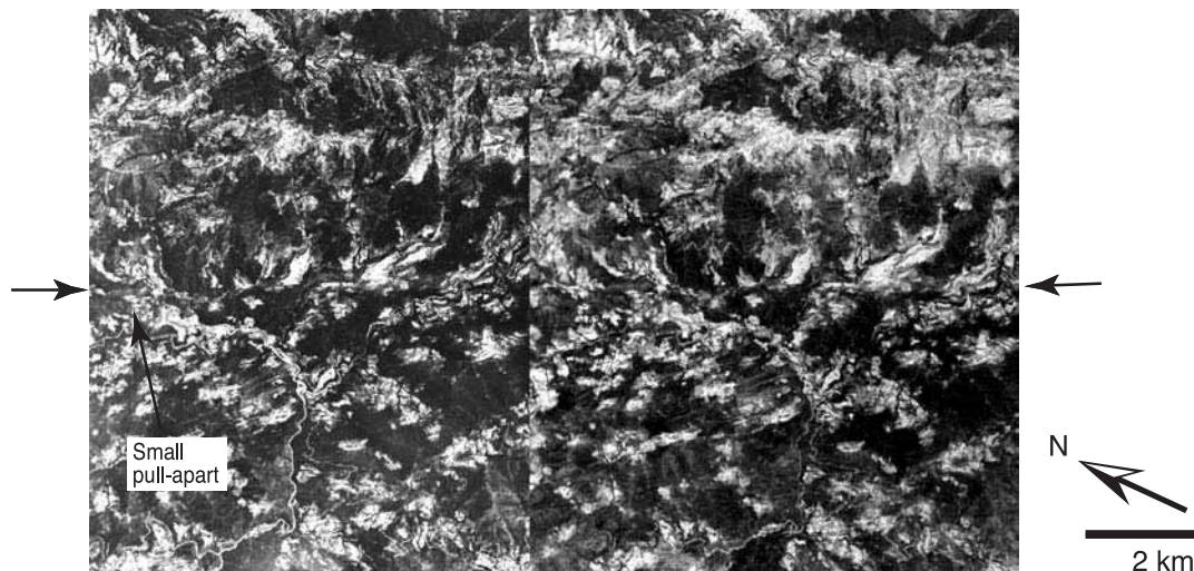
Fig. 12. Stereo-pair of satellite photos showing right-lateral stream offsets along NNW-SSE trending Taksal Fault between Banet and Chewag villages (refer to fig. 3 for location). The fault has displaced along it Tertiary strata as well as Quaternary sediments. Along with the streams, younger terraces are seen displaced right laterally along the fault. Right stepping along the fault has resulted in formation of small pull-apart near Chewag village.
