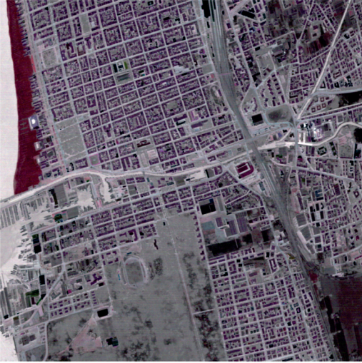
Fig. 4. MIVIS composite image acquired over Viareggio and obtained mapping the 100th channel as red, the 95th channel as green and the 93rd channel as blue.
