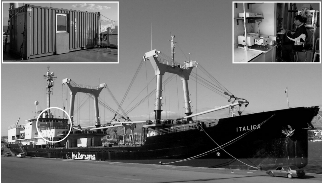
Fig. 1. Main picture: RV Italica; ELF and the ancillary instruments are housed in a container (inside the circle). Left insert: external view of the container; note on the left of the container the box accommodating the mirror for water surface observation. Right insert: internal view of the container; ELF and the spectrofluorometer are visible behind and on the left of the operator, respectively.
