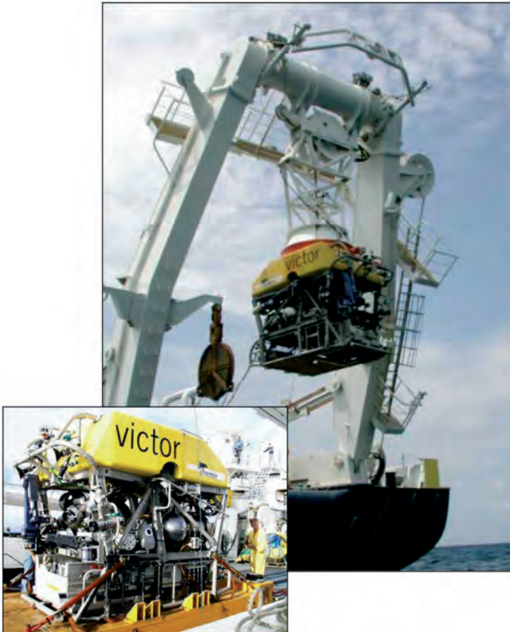
Fig. 2. The French deep-rated ROV Victor 6000 built and managed by IFREMER (see also table II). A detailed view of the ROV is shown in the bottom-left corner.
