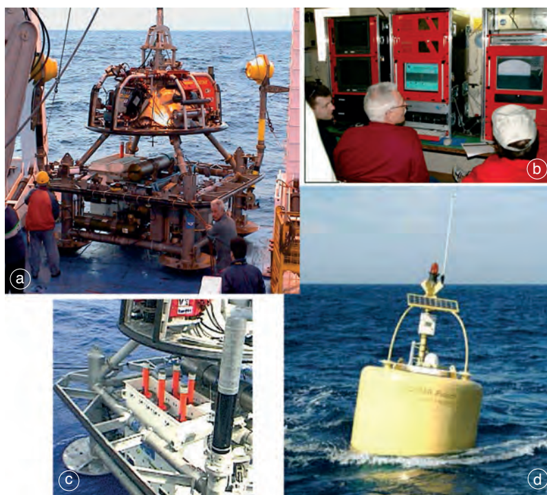
Fig. 9a-d. The complete GEOSTAR sub-systems: a) Bottom Station, which includes DACS, power supply, underwater acoustic communications and scientific payload, with MODUS on the top; b) MODUS ship-based remote control system; c) surface communication buoy (GEOSTAR-2 configuration); d) five MESSENGERS within the Bottom Station, the orange ARGOS antennas are visible (see also Favali et al. , 2006).
