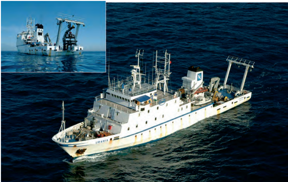
Fig. 1. R/V Urania , a medium-size vessel (overall length: 61 m; gross tonnage: 1100 t) owned by CNR and managed by SoProMar. The top-left corner shows the ship during the launch of a GEOSTAR-class observatory.
