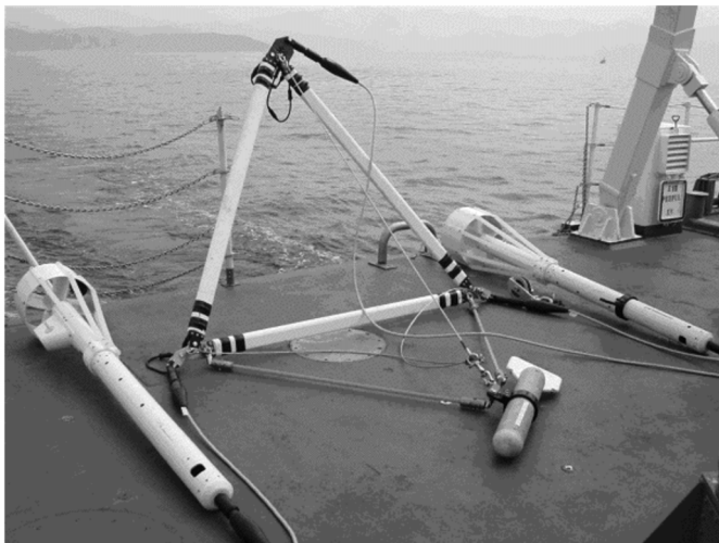
Fig. 2. Instrumentation used for the transverse gradiometric array; the two sensors, the ballast and the triangular frame are visible.
