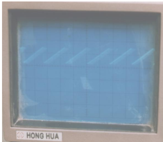
Saw-tooth Waveform, Frequency =125 kHz
