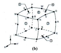
Fig.3, Element Geometry; (a) Plane 42, (b) SOLID 95.
