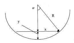
Fig.1, Geometry of Cam-Follower Contact Near Circular Limit.
