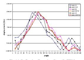
Fig.14. Deflection Function Cam (2) FEM.
