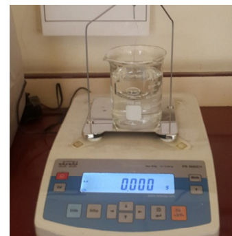
Fig. 13. Sensitive Libra used (division 0.001g) with Hang system.
