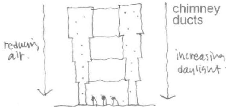
Image from the initial workshop of the ventilation air supply and window concept
