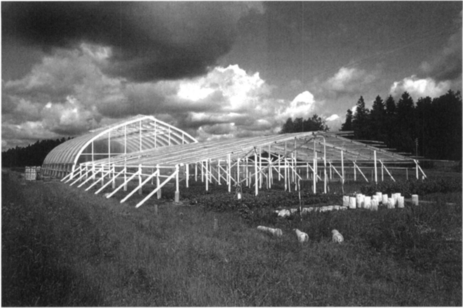
Fig. 1. The greenhouse built on the experimental field in order to elevate the temperatures continuously by 3°C, and the adjacent open field, covered with the same material as the greenhouse.
