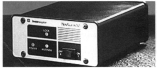
Fig. 75. (a) The DGPS/DR (Differential GPS satellite navigation with DR backup) receiver (front view, size c. 150x50x250 mm) and the DR module and (b) the RTCM-radio beacon (c. 150x75x250 mm). (Courtesy: Trimble Navigation Inc)
