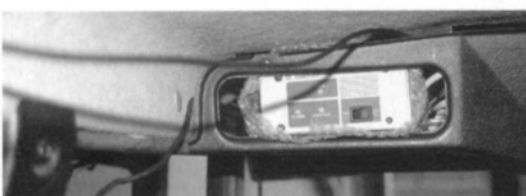
Fig. 77. The DGPS/DR installed in an agricultural tractor in 1993. (a) the GPS/DR module and (b) the RTCM receiver installed in tractor cabine. (Photos: Markku Hirvenoja).
