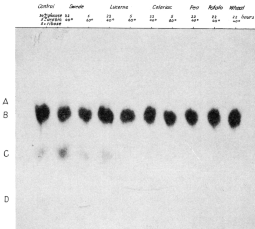
Fig. 1. Paper chromatogram of sugars in the starch hydrolysates of some plant materials. A galactose, B glucose, C arabinose, D ribose.
