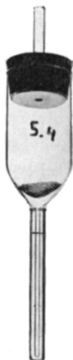
Figure 1. Glass tube with its capillary part, rubber stopper with hole, frosted glass wedge and brass gauze.
