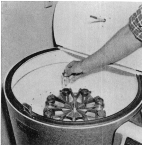
Figure 3. An International size 2 model V centrifuge used in the centrifuging of heads.
