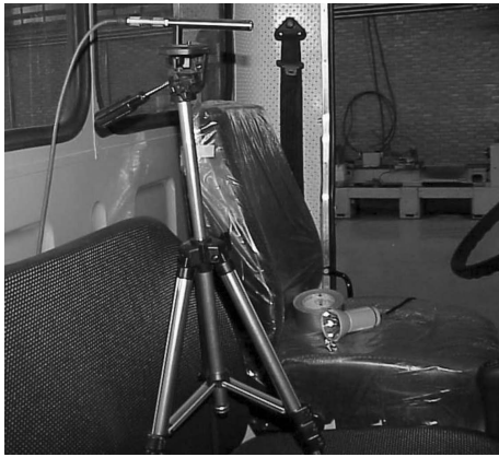
Fig. 8. Position of the microphone inside the cabin.
