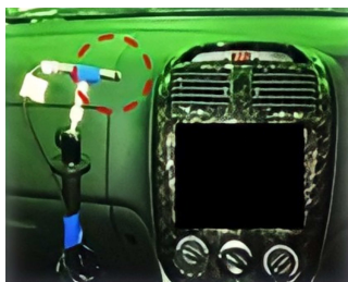
Fig. 4. Microphone arrangement at the center outlet of the vehicle HVAC system.
