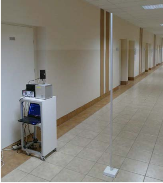
Fig. 25. Location of the rotary base with the sonar module in relation to the post.
