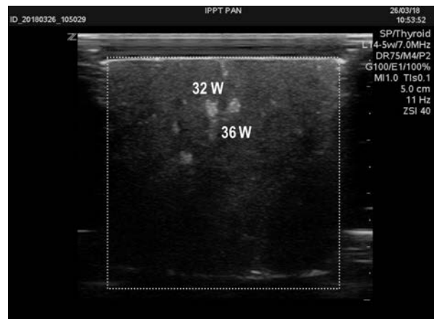
Fig. 7. Ultrasound image of the axial section ( xz ) of the tested tissue sample placed in the cylindrical chamber after its exposure to two parallel, spaced by 4 mm, HIFU beams with the acoustic power of 32 W and 36 W.
