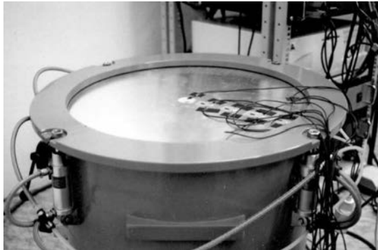
Fig. 1. Circular plate with sensors and actuators.
